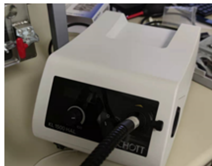
Fig. 2.4 Schott KL 1500 Halogen lamp wavelength range – visible light, 380-750 nm.
