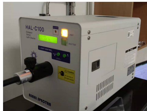
Fig. 2.5 Solar Simulator HAL - C100 wavelength range 400-1100 nm.
